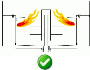
**CORRECT DRAFT:** the tips of the flame are at the same level as the top of the "S" tube
