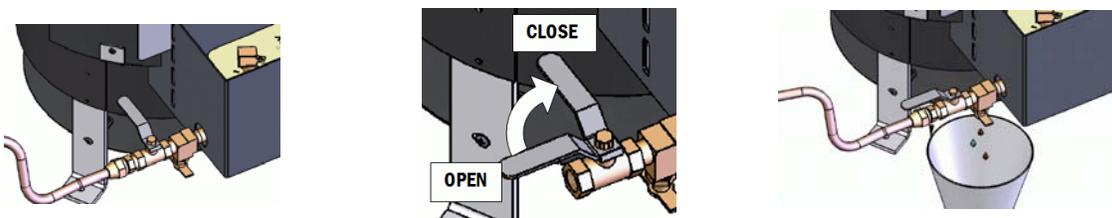
7c. **USING A SOLID FUEL LINE** Connect the solid fuel line to the heater. Turn the ball valve lever to the OPEN position and open the fuel drain valve. Start the fuel flowing from the fuel tank and wait until fuel flows in a steady stream from the drain valve. Catch the fuel in a separate container, then close the fuel drain valve. The fuel line is clear of air.
