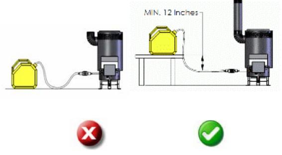
3. Before operating the heater, position the fuel source a minimum of 12" above the level of the fuel inlet to the heater.
