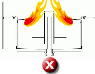
**LOW DRAFT:** The tips of the flame are at a level higher than the top of the "S" tube.
