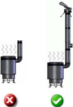
4. **DO NOT** operate the heater without both a complete exhaust stack (see page 2) in place and correct draft conditions (see below). Excessive carbon will form in the fuel up-tube and will have to be cleaned out for the heater to function correctly.
