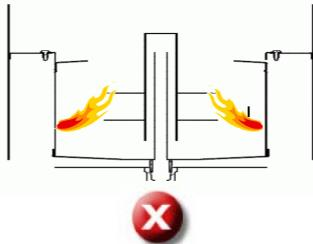
**HIGH DRAFT:** The tips of the flame are at a level lower than the top of the "S" tube.
