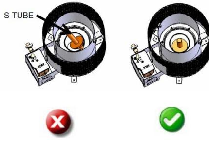
2. During shipping, the S-tube may become dislodged from the center fuel up tube. If the S-tube has become dislodged, which can be seen through the glass on the lid, the top of the heater must be removed to position the S-tube over the fuel up-tube.
