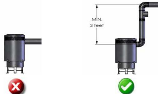
6a. **DO NOT** connect horizontal exhaust stacks directly off the heater (Expedition, Prospector). The heater will not operate correctly and will not stay lit. All heaters (except Trekker) require a 90 degree exhaust elbow and a minimum three foot vertical rise before further elbows and exhaust stack lengths are added.
